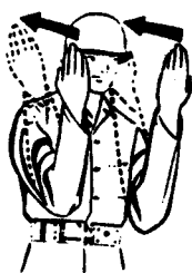
Move ahead. Arms a little aside, palms facing backward and repeatedly moved upward-backward from shoulder height. Indicate the speed desired of the aircraft by rapidity of arm motions (STANAG 3117).
